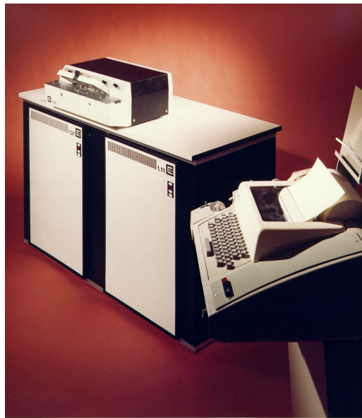
A basic Modular One system with a paper tape reader and an ASR33 teletype for simple I/O.
