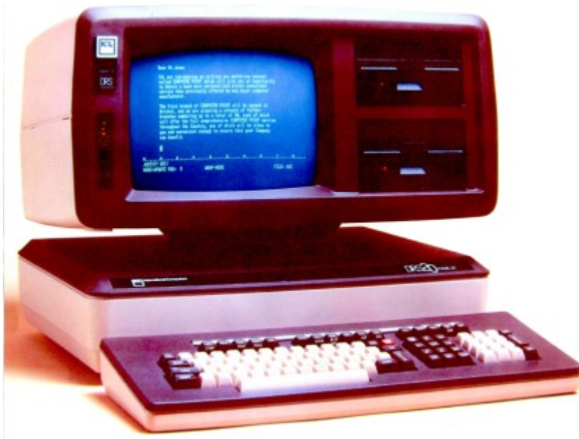
Fig. 2 A DRS20 model 20 Function Processor system of 1982: The photo shows the distinctive keyboard design and the double 5¼” mini-diskette drive within the display cabinet.
