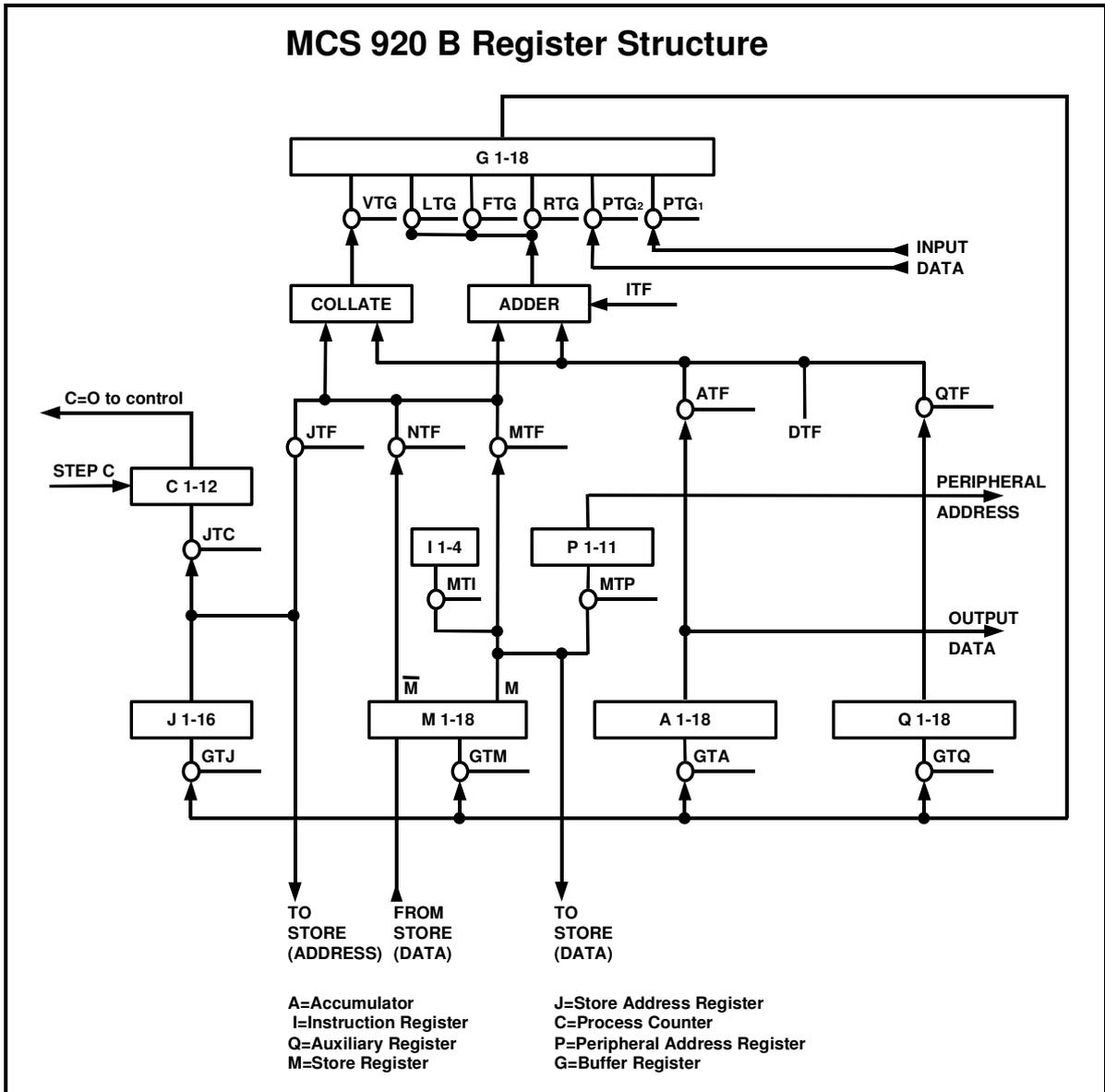
*Of these registers, the only ones which convey information from one instruction to the next, and so are of interest to the programmer, are the A-Register (or Accumulator) and the Q-Register (or Auxiliary Register).*
