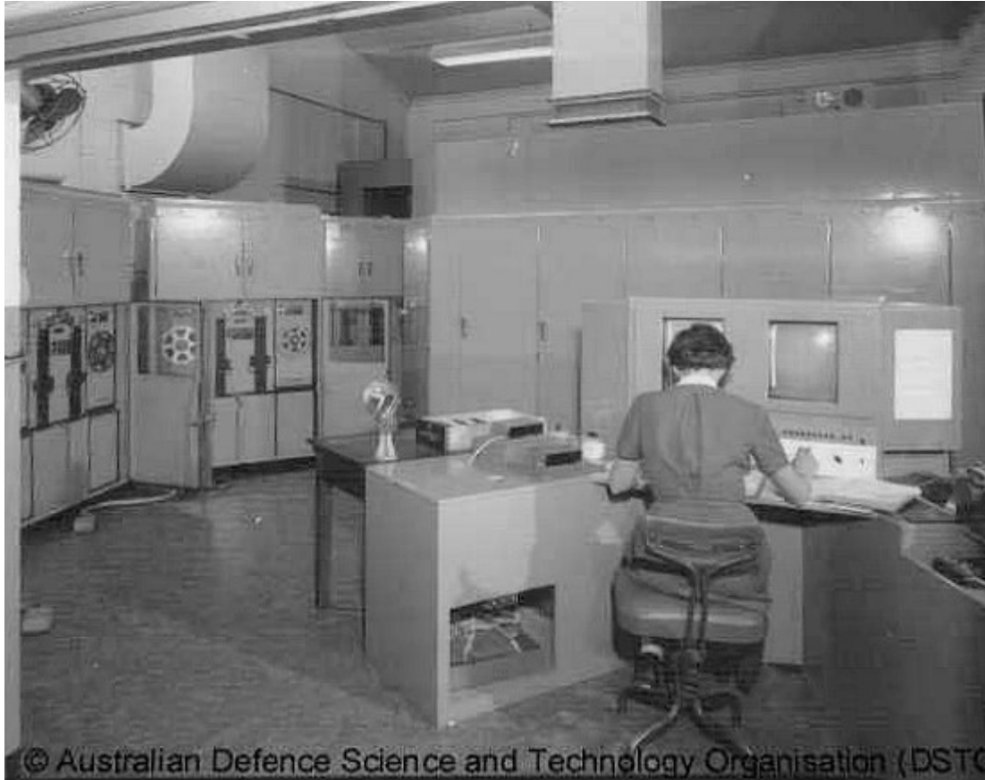
WREDAC, showing the replacement console designed and built by WRE engineers. Reproduced by courtesy of the Defence Science and Technology Organisation, Australia
