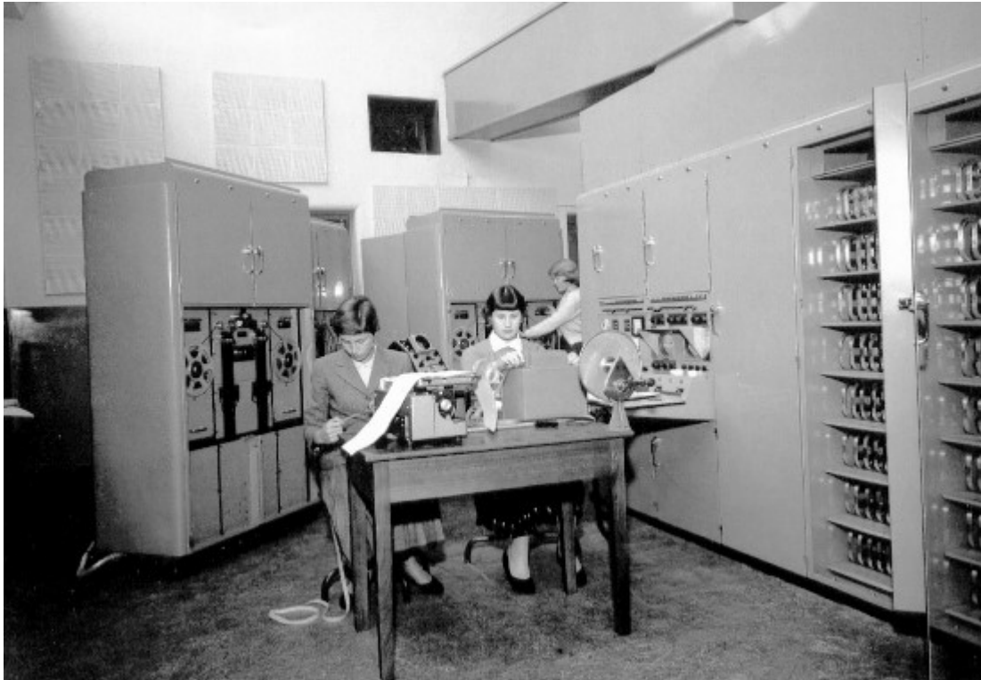
Above: Operating the WREDAC punched paper tape equipment. Left to right: Barbara Lane (later Biggins), Bronte Walter (later Morrison), and Robin Fleming. The WREDAC (403) cabinets and original console are on the right.
