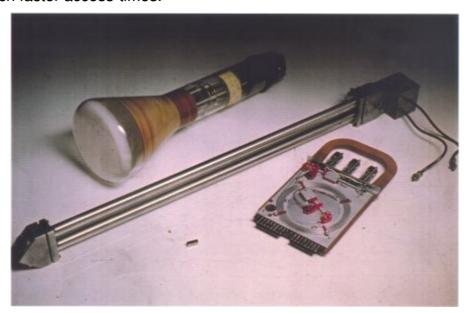
The upper left device in the photo is a CRT *Williams-Kilburn* storage tube from a Ferranti Mark I computer. In the centre is a mercury delay line from an English Electric DEUCE computer, where acoustic signals are transmitted down one tube and reflected back along the other tube. At the right is a package from a Ferranti Pegasus computer containing a nickel delay line register.
